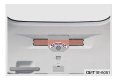
Warning triangle is located on the boot door panel, turn the retaining clamp counterclockwise to remove it.
