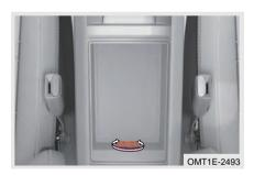
Place necessary items (For example: Canned drinks) in the auxiliary fascia armrest box to perform A/C cooling operation. Rotate inner button of armrest box to cool the necessary items.
