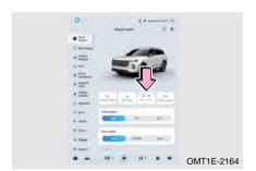
Click vehicle window lock button throughAudio System - Vehicle Center -Quick Control to turn on/off Child-protector Lock function.
