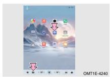
■ Entering panoramic view monitor When vehicle is in READY state, and vehicle speed is 18 mph (30 km/h) or less:
