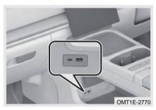
USB port is located on the lower front part of auxiliary fascia console.
