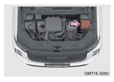
Step 3: Remove the engine compartment fuse box cover to check or replace the fuse.
