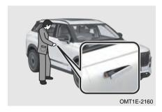
Step 2: Pull the door handle, insert the mechanical key into the keyhole inside the door handle, turn clockwise to lock the door, counterclockwise to unlock the door.
