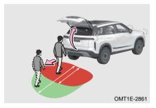
While vehicle power is switched to OFF mode or vehicle is started remotely, four doors are closed, approach to the back (red area) of vehicle when carrying smart key on your person and wait 3 seconds, after indicator signal lights come on, take a step back (green area), power boot door opens.
