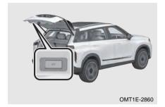
Method 1: When the power boot door is open, adjust it to your desire height; long press " " switch until the vehicle gives a light prompt, and the power back door opening height is set successfully.
