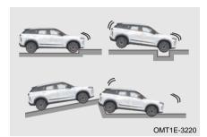
The driver airbag, front passenger airbag, front side airbags, curtain shield airbags and front middle airbag may also deploy if a serious impact occurs to the underside of your vehicle.
