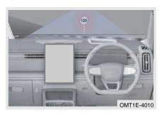
After SLA detects speed limit sign information on road in front and combines the information with speed limit information of navigation system, "" indicator in instrument cluster remains on, If the speed exceeds the current speed limit, the driver will be alerted by flashing/sounding the speed limit icon.
