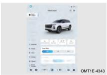
With vehicle in READY state, click Eco/NORMAL/Sport button in Audio System - Vehicle Center - Quick Control to switch the driving mode; The corresponding mode indicator on instrument cluster comes on, accompanied by voice reminder, to prompt you that driving mode is switched successfully.
