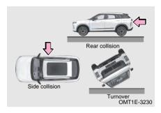
The driver airbag, front passenger airbag and driver knee airbag will usually not deploy if the vehicle is involved in a side or rear collision, if it rolls over, or if it is involved in a low-speed frontal collision.
