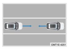
Activation conditions: The vehicle shift position is not in R and the vehicle speed is 9 mph (15 km/h) or more.
