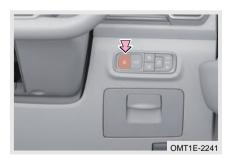
Step 1: The vehicle is parked, long press " " button and instrument cluster displays "It is ready to refuel, please refuel" message, and fuel tank cap unlocks after the pressure relief is completed;
