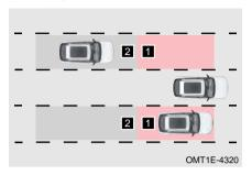
When speed increases to 9 mph )15 km/h) or more, BSD system enters activating; When speed is decreases from more than 9 mph (15 km/h) to 6 mph (10 km/h), BSD system enters pre-activating.
