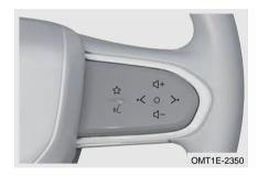
Customization button "☆": This button can be customized in audio system - Vehicle Center - Vehicle Settings.
