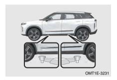
Make sure that the vehicle is on the correct jacking point to avoid damage to high/low voltage cables or power battery when the vehicle is lifted.
