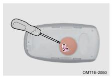
Step 2: Pry off battery cover and battery using a flathead screwdriver with the tip taped;
