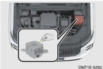
Step 3: Remove front compartment fuse box cover, refer to fuse box location diagram at fuse box upper cover, pull BMS fuse out by a fuse remover and disconnect the BMS module power.
