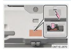
Back door cannot be opened when battery is depleted or under similar conditions. In this case, the back door can be opened with emergency device switch.
