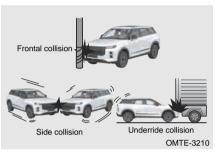
The driver airbag, front passenger airbag and driver knee airbag may not deploy if the front of vehicle hits a telegraph pole, goes under a truck, or if the vehicle is involved in an sideways collision.
