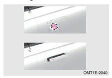
Bring smart key and touch the sensing area of hidden door handle. After system recognizes unlocking signal, the hidden door handle extends automatically, then indicator signal light flashes twice and the door is unlocked.
