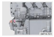
With the engine stalling and cooled down, check the oil level with the dipstick.
