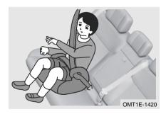
For larger children that cannot fit in a child restraint system with a high back, they may occupy a second row outboard seat using a booster seat. either attached to the lower anchorage points or belted, as described in the instructions provided bv the child restraint system manufacturer.
