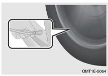
Step 3: Tighten the junction valve of the automatic inflation tyre repair liquid to the tyre valve;
