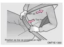
To adjust the seatback angle, sit up straightly and well back in the seat. Position the lap belt as low as possible on your hips — not on your waist, then pull the shoulder section upward so that it comes fully over the shoulder, but does not come into contact with the neck or slide off the shoulder.
