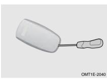
The mechanical key built into the smart key can be used to lock/ unlock doors in emergency after prying off smart key cover using a flathead screwdriver with the tip taped and taking out mechanical key. After using, return it to original place for easy-to-carry (for details, refer to "Door").
