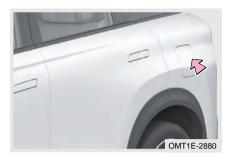
Step 2: When the fuel cap is unlocked, the fuel tank cap will pop up outward while pressing it;
