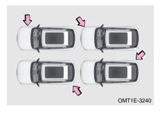
The side airbags, curtain shield airbags and front middle airbag may not deploy if the vehicle is subjected to a collision from side, the rear part of the rear tyre or a side collision at certain angles to the vehicle.
