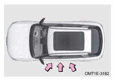
The vehicle is subjected to a strong side impact, and the side collision sensors detect an impact severe enough to cause the side airbags, curtain shield airbags, and front middle airbag to deploy.
