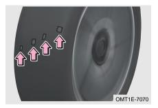
Check the tyre tread by tread wear mark. When tread wear reaches its limit, tread will be in the same plane as the wear band. If such condition occurs, the tyre performance and safety will be seriously impacted, and replacement is necessary.
