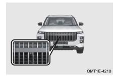
Installation position of front camera: located at intake grille of front bumper.
