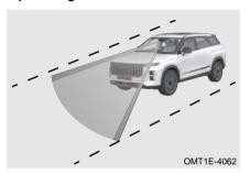
When vehicle speed is no less than 40 mph (65 km/h) and vehicle target is monitored, ELK enters standby status.
