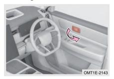
When doors are unlocked, pull door inside handle simply to open door. When doors are locked, pull door inside handle for the first time to unlock the door, and pull it again to open the door.
