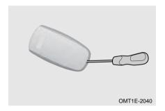
Step 1: Pry off smart key cover using a flathead screwdriver with the tip taped;
