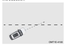
When vehicle speed is no less than 40 mph (65 km/h) and lane line is recognized, LDW enters standby status.
