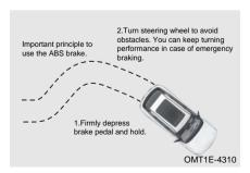
ABS does not function during normal braking and it will be turned on immediately only during sudden braking (brake pedal pulsates with noise, ensuring brake performance and steering performance, if the space is enough, the vehicle can also avoid obstacles). Never release brake pedal in this case.
