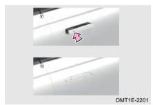
Bring smart key and touch the sensing area of hidden door handle. After system recognizes locking signal, the hidden door handle retracts automatically, then indicator signal light flashes once and the door is locked.
