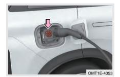
Step 5: Press the switch button on power strip and wait for red indicator to remain on, which indicates that the external discharging device is successfully connected; after the external discharging device is successfully connected, the vehicle starts to discharge, and the vehicle displays the discharge information;
