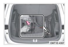
When abnormal lock fault occurs in electronic lock of the charging gun or discharging gun, the charging gun and discharging gun can be manually unlocked with electronic lock cable.
