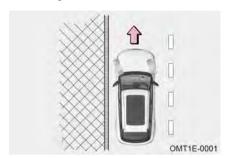
If there is a curb on the roadside, turn the steering wheel to the left to ensure that the front part of the front left wheel is close to or against the curb, to prevent the vehicle from sliding forward down the slope, then apply the parking brake.
