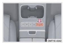
With vehicle in READY state, press EV/HEV button to switch the power mode; The corresponding mode indicator on instrument cluster comes on to prompt you that power mode is switched successfully.
