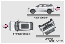
The side airbags, curtain shield airbags and front middle airbag may not deploy if the vehicle is subjected to a front or rear collision, turnover or low speed side collision.
