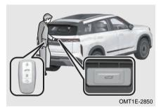
Method 1: With central control lock unlocked, approach the back of vehicle and press exterior switch, on the boot door, turn signal lights will come on and power boot door will be opened/closed.
