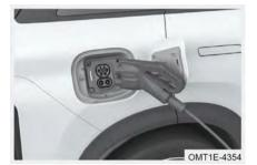
Charging cable has anti-theft function. After inserting charging cable and entering full power charging or when doors are locked. charging aun will be locked automatically.
