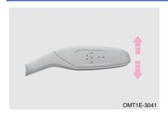
P gear: When the vehicle is stationary, depress the brake pedal and the shift lever is not in P. Press the button on the right side of column shift switch to shift the shift lever to P.
