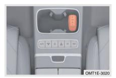
Lay smart key in auxiliary fascia console storage box with front side facing up (as shown in figure), depress brake pedal to start vehicle, and "READY" green indicator on instrument cluster remains on.
