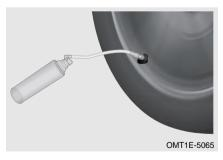
Step 4: Turn the red valve clockwise and place the bottle upside down to start inflating the tyre;
