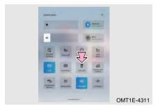
Turn vehicle power supply to ON mode, slide down from the top right edge of the audio system screen, click ESP OFF switch to turn off ESP; click ESP OFF switch again to turn on ESP.
