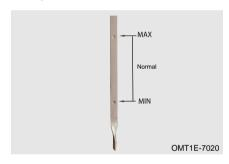
Put a cloth under the dipstick to avoid oil spilling onto engine or vehicle body.
