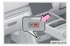
Step 3: Connect USB port and phone using original data cable;
