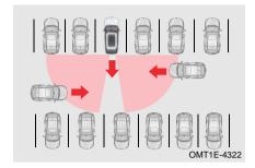
Shift the shift position to R and vehicle speed is less than 9 mph (15 km/h), rear traffic crossing anticollision system is activated; In other gear positions, system is in standby status.
