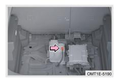
Step 1: Turn vehicle power to OFF mode, and connect jumper cables:
