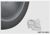
Step 2: Shake the automatic tyre filler well before use, and then tear off the safety belt of the junction valve;
