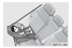
A rearward facing child restraint is installed to face to the rear of the vehicle. Only install a rearward facing child restraint on the front passenger seat if the airbag is OFF. It is recommended children use a rearward facing child restraint system up to 4yrs old.
