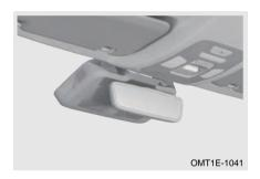
When driving at night, the light sensor installed in front/rear of the inside rear view mirror automatically detects the reflected light from the headlights of vehicles behind and automatically adjusts the lens angle to reduce the reflected light from the headlights of vehicles behind.
