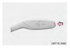
Fully depress the brake pedal, press P button on shift lever to shift to P, the parking brake function can be applied automatically by EPB system.
