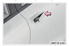
Step 1: Press and hold the front area of the driver door outside handle to open the hidden door handle.
