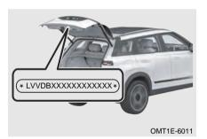
Vehicle Identification Number (VIN) label is located on boot door as shown in the illustration.
