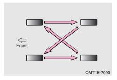
To equalize tyre wear and extend tyre service life, we recommends that you should rotate your tyres approximately every 6214 miles (10,000 km) (best adjustment range is 3107 - 4349 miles (5,000 - 7,000 km); the tyre rotation cycle may vary according to your driving habits and road surface conditions.
