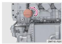
Step 1: Turn the engine oil filler cap counterclockwise to open it;
