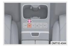
With vehicle in READY state, press " button to cycle through the driving modes; The corresponding mode indicator on instrument cluster comes on, accompanied by voice reminder, to prompt you that driving mode is switched successfully.
