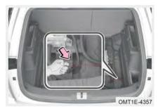
When abnormal lock fault occurs in electronic lock of the charging cable or discharging cable, the charging cable and discharging cable can be manually unlocked with electronic lock release cable.
