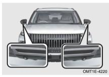
Installation position of left / right cameras: located at the bottom of left / right outside rear view mirrors.
