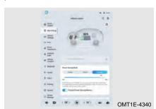
With vehicle in READY state, turn External Discharge to ON/OFF on New Energy screen. Before unplugging the discharging gun, it is necessary to turn External Discharge to OFF.
