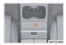
In case of vehicle failure or traffic accident etc., please turn on the hazard lights to warn other vehicles, so as to avoid the secondary accident.
