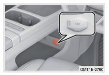
Front power outlet is located on the lower front part of auxiliary fascia console.
