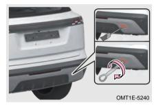
Step 1: Use a screwdriver with its tip taped to remove the rear towing eyelet hole cover.
