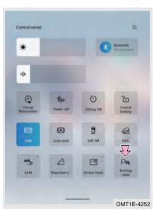
When vehicle is in READY state, slide down from the top right edge of the audio system screen, click parking radar button, parking radar system turns on; when shift lever is not in R, click parking radar button again to exit.
