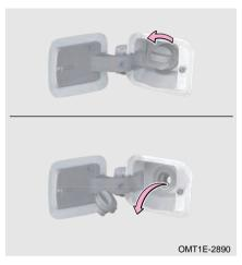
Step 3: Turn fuel filler cap counterclockwise to remove it:
