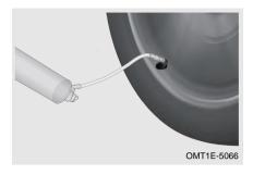
Step 5: After the automatic inflation tyre repair liquid is filled, close the valve counterclockwise and screw out the junction valve. Then immediately drive for 6 miles (10 km) or more to complete the repair. Please go to authorized service centre or professional tyre repair shop for repair and replace as soon as possible.
