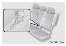
When inserting the small tab into the small buckle of left side of the second row seat, use a screwdriver with its tip wrapped with tape or similar object to press the position shown in illustration and pull out the small tab.
