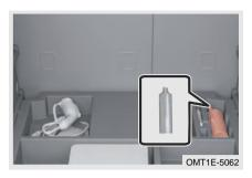
Step 1: Open boot door, lift the luggage compartment carpet and take out the automatic inflation tyre repair liquid;
