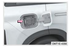
The indicator light strip is located inside the charging port cover.
