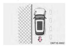
If there is a curb on the roadside, turn the steering wheel to the right to ensure that the rear part of the front left wheel is close to or against the curb, to prevent the vehicle from sliding back down the slope, then apply the parking brake.
