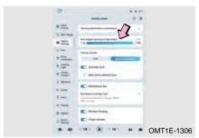
Method 2: With vehicle in READY state, set the opening height by Audio System - Vehicle Center - Vehicle Settings.
