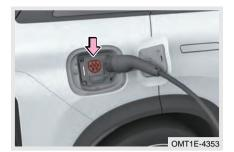
Step 4: Open the boot door and take out the charging device, then insert the three-pin plug into a standard power socket (only using on-board charging gun is applicable to this step). If AC charging pile is used for charging, please skip to step 5 directly;
