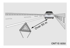
Place the warning triangle at a distance of more than 50 m behind the vehicle on a normal road.
