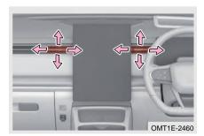
Move center outlet adjustment lever up, down, left or right by hand to adjust direction of airflow.
