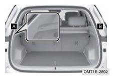
Pull the luggage curtain to the slots of point A and point B to secure it, and confirm if it is secured properly.
