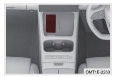
While vehicle power is switched to ON mode, the wireless charging starts to work after putting the mobile phone in wireless charging sensing area, and the audio head unit displays " (1)) ". The audio head unit displays " (1)) " after charging is completely.
