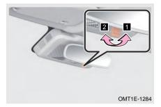
Before driving at night, adjust the inside rear view mirror lever to the anti-glare position, which can reduce the reflected light from the headlights of vehicles behind.
