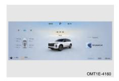
When vehicle speed is not lower than 15 mph (25 km/h), if TPMS has not received radio-frequency signal from one or more sensors after several minutes, TPMS will send system malfunction warning, " (!) " yellow indicator on instrument cluster will blink for tens of seconds and then remains on, "Abnormal Tyre Pressure, Check" will be displayed for several seconds and then turned off, which can be checked on tyre pressure display screen.
