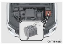
Step 3: Check the fuse according to fuse and relay location distribution diagram, use the puller to remove the possible faulted fuse;
