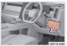
Step 3: Remove instrument panel lower left protector to inspect or replace fuse.
