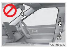
Do not attach anything to areas such as the door, windshield glass, side door glass, A pillar, B pillar, C pillar, roof side rail and assist grip.
