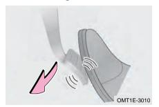
With vehicle powered on, carry the smart key on your person and enter the vehicle, depress brake pedal to start vehicle, and "READY" green indicator on instrument cluster remains on.
