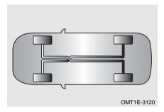
The brake system adopts X type arrangement, double circuit brake system; The system is a hydraulic with independent system two subsystems. If one of subsystems fails, the other system can still perform brake function. However, the brake pedal should be depressed more firmly than usual braking distance increase, and the brake system malfunction indicator remains on
